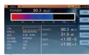
DVB-T signal measurement
